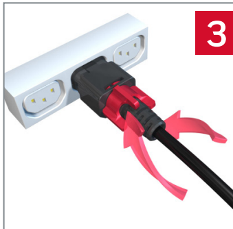
3 Push and tighten the nut to initial resistance, then add 1/4 to 1/2 turn to secure. (Do not over-tighten)
