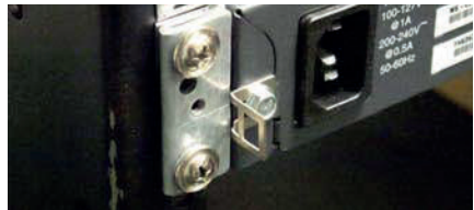
Figure 2 – Installation of Tie Wrap Retainer
